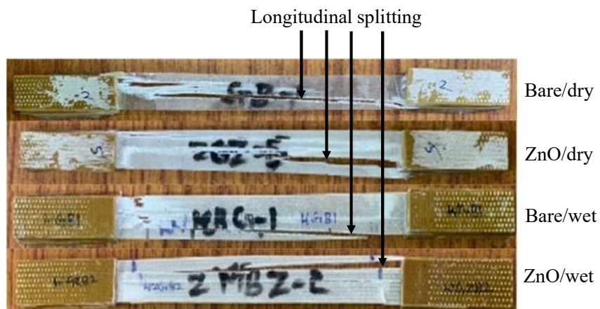
Figure 2: Failure modes of glass composites under tension test
